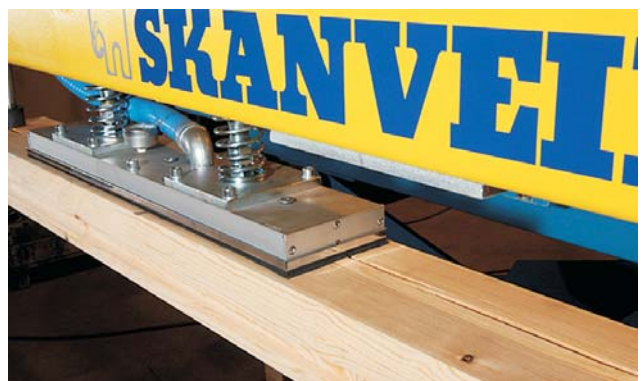
The suction box device feeding planed logs to further processing
